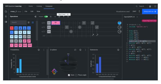
We see the first qubit has probability amplitude 0.5 for  $\alpha$  and 0.866 for  $\beta$ . The probabilities then are 25% resp. 75%.
