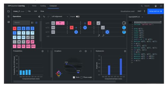
We see that the state vector has only two components in the first entry, the last qubit, with probability amplitudes 0.5 for qubit  $|0\rangle$  and 0.866 for qubit  $|1\rangle$ . This is the state the first qubit was in at the beginning of the process.
