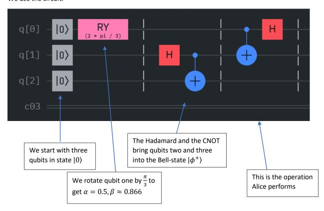
We check the circuit step by step. Note that in the pictures we have IBM-notation, the upper qubit is right.
