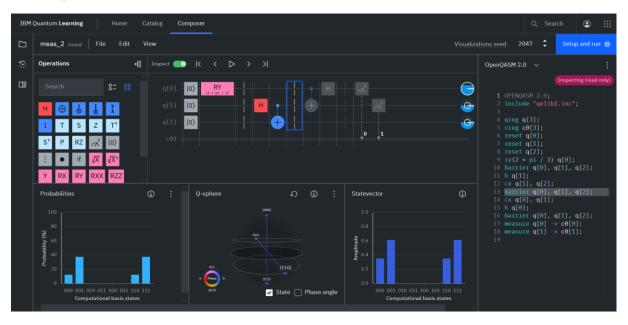
We produced the Bell-state  $|\phi^+\rangle$ , the lower two qubits are in the state  $\frac{1}{\sqrt{2}}(|00\rangle + |11\rangle)$ . Note that the probability amplitude is mixed up with the factor belonging to the first qubit.
